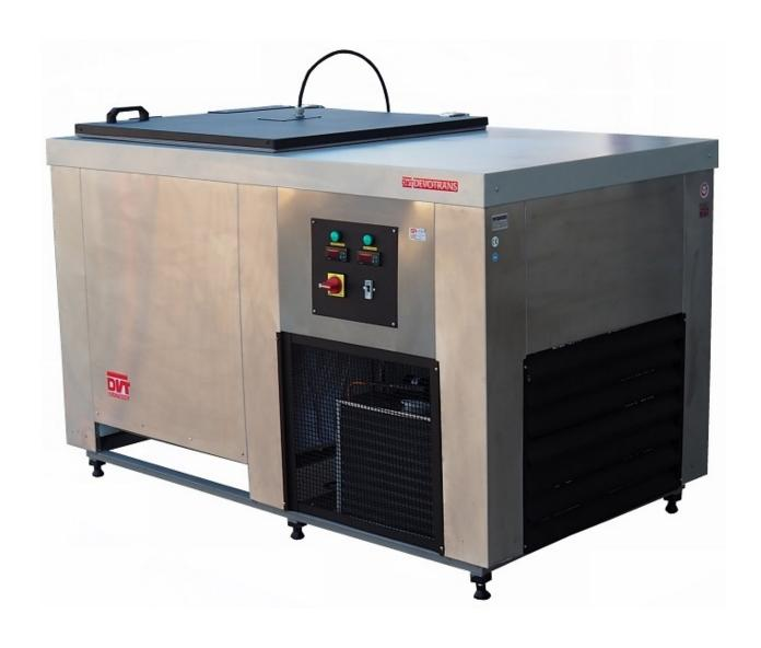
FOR TESTING BEHAVIOUR OF PRODUCTS IN COLD ENVIRONMENT
